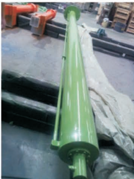
6550mm hydraulic cylinder uses 19 series
