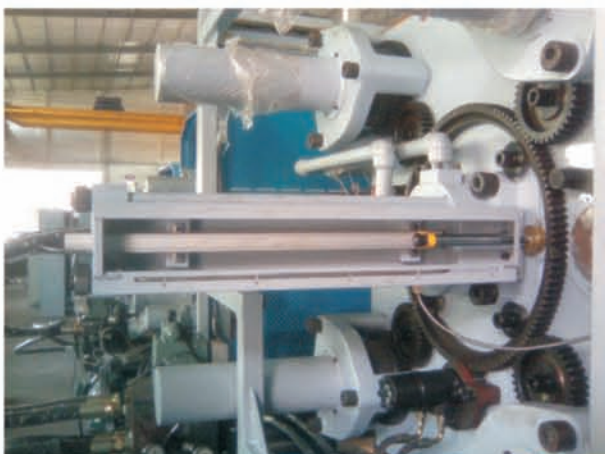
Mold closing at die-cast machine. injection speed at 10m/s
